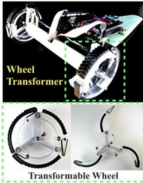
Fig. 1. New type of transformable wheel and Wheel Transformer.
