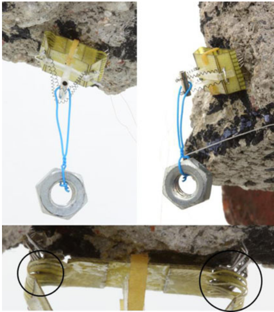
Fig. 1. Buckling gripper—dimensions of 15 mm \times 10 mm \times 6 mm and weight of 140 mg—attached to a cement block weighing 3 g (note that the tested cement block had surface waviness of 583.93 \mu m, which is more than six times surface roughness of normal concrete). The flexures of each spine show different bending angles since they adapt to the wavy surface (see the circles in the figure).
