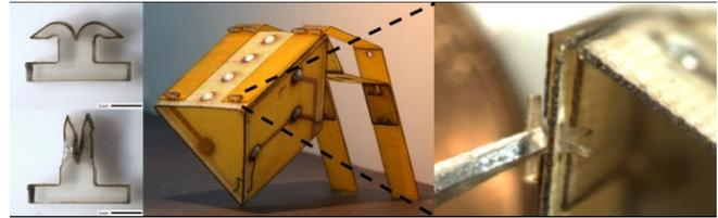
Fig 1. Assembly of legs with the body of meso-scale flea robot, using the anchor shape SMP rivet fasteners.
